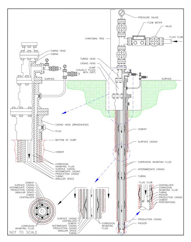
Figure 5: Typical Injection or SWD Well
